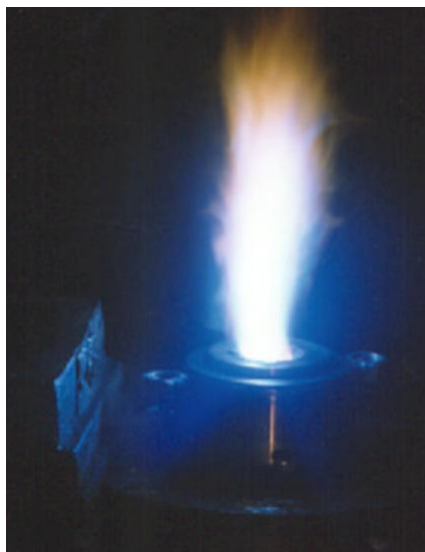
Figure 2: Plasma Torch producing high temperature plasma
